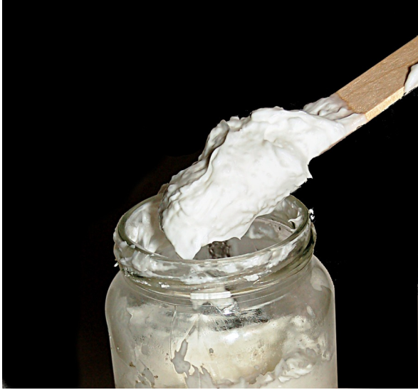
Cold wax paste made with mineral spirits and white beeswax prill.
